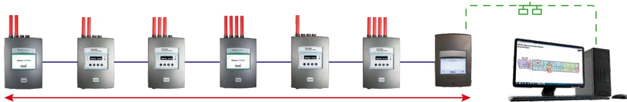
Maximum 98 Protac air sampling detectors on RS485 wired network Maximum 1.2km RS485 network length with one ADRDP (can be extended using multiple ADRDPs)
